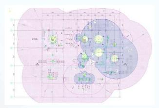
Hazardous areas are classified into zones based on an assessment of the frequency of the occurrence and duration of an explosive gas atmosphere, as follows:
